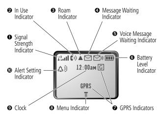
**O** Signal Strength Indicator Shows the strength of your phone's connection with the network.
