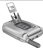
4 Close the SIM card door and slide it up to lock the SIM card in place.
